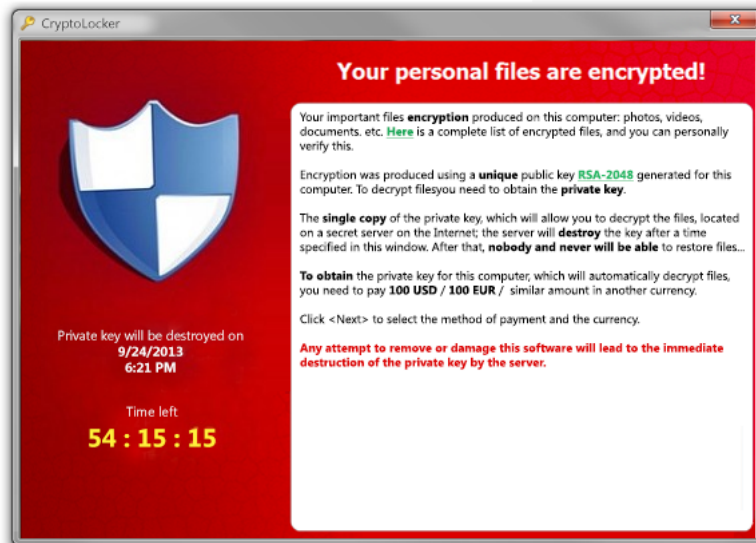
Figure 2: You don’t want to see this Classic Ransomware operation - after the malware is in place, a unique encryption key is generated for each computer infected and is used to encrypt data on the machine. If the ransom is not paid within the allotted time the files are lost forever.
